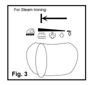
Steam is produced as soon as the iron is held in the horizontal position. Steam will stop coming out when the iron is put on its heel in a vertical position or by turning the steam control dial to "0".
